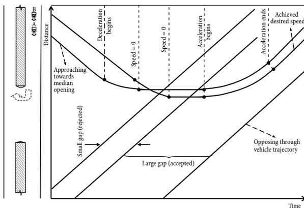
Fig. 5. Time–distance diagram for parallel SM
