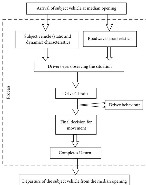
Fig. 1. Flow chart of decision making for U-turning process
