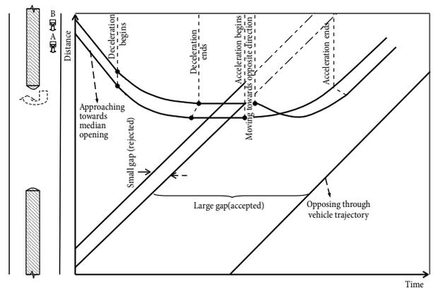
Fig. 6. Time–distance diagram for stream lined SM
