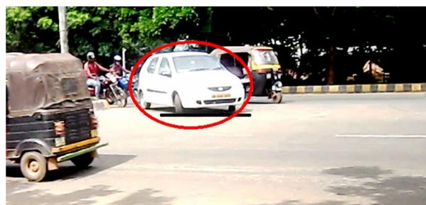
The front bumper of the U-turning Vehicle arrives at reference line ( $t_0$  – service delay starts)
