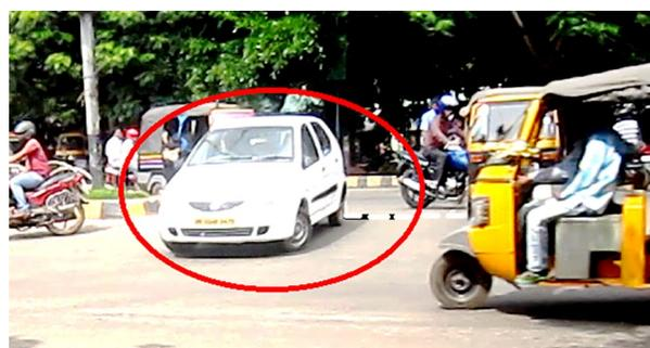
The rear bumper of the U-turning vehicle departs from reference line ( $t_d$  – end of service delay or initiation of merging)
