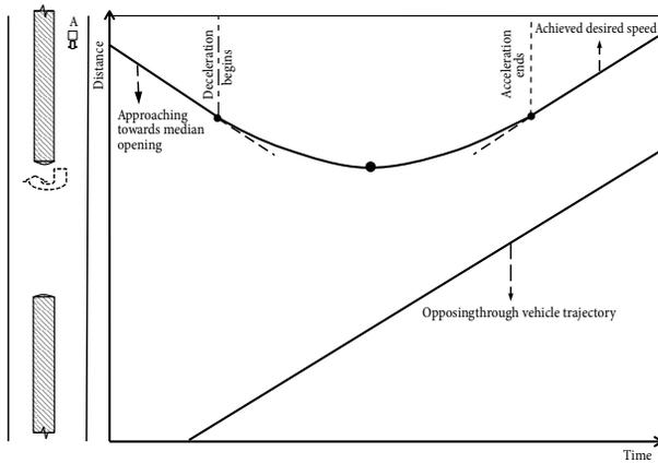
Fig. 3. Time–distance diagram for free merging
