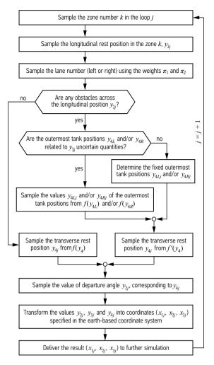
**Fig. 7.** A flowchart of the simulation step *j*
