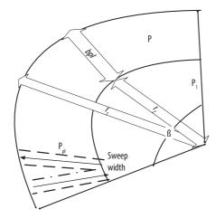
Fig. 4. Values to calculate the number of sweeps
