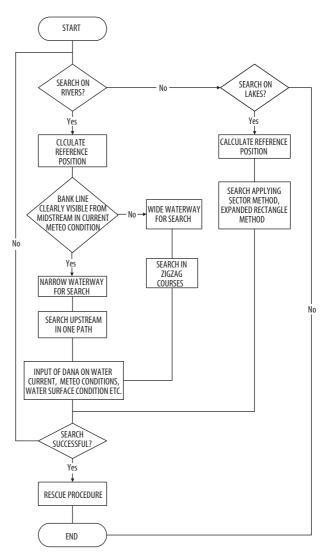
**Fig. 10.** General search algorithm for the rescue of a drowning person on inland waterways
