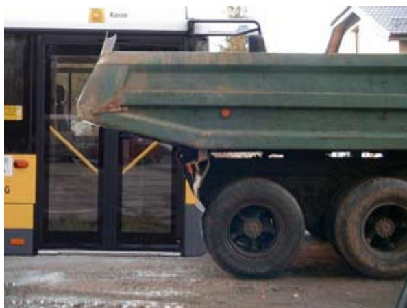
Fig. 8. View of the wide trailer (drawing alongside a car) with invisible (covered by the trailer) mirrors
