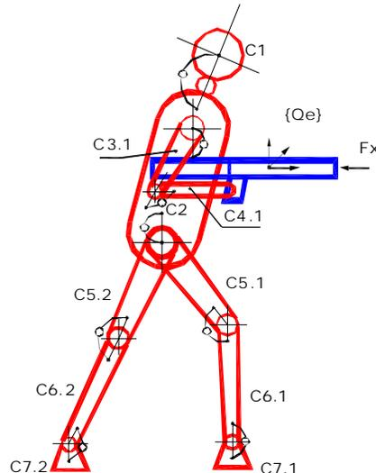
Fig. 4. Diagram of forces acting on the extinguishing device and fireman
