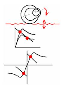
**Fig. 20.** Illustrative figures of three basic types of excitation of wheelset torsion dynamics
