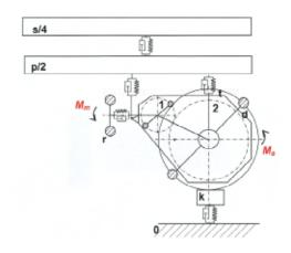
Fig. 11. The model of wheelset drive by hollow rotor
