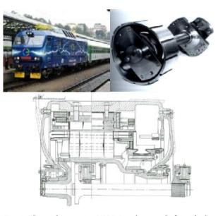
Fig. 3. Electric locomotive SKODA with jount shaft inside the hollow rotor and a detail section
