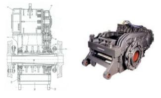
Fig. 7. Integrated unit with auxiliary hollow shaft with brake discs (ICE 1, ICE 2)
