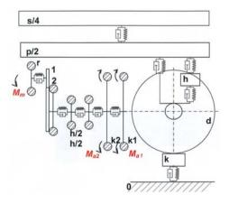
Fig. 13. The model of wheelset drive by hollow joint shaft
