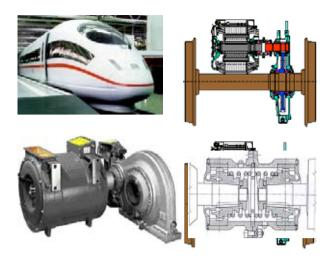
**Fig. 4.** High speed train ICE 3 – drive by outside location of cardan shaft and special tooth clutch
