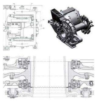
Fig. 6. Integrated unit IGA and its installation in bogie frame of locomotive DB 120; a detail section of complicated joint of hollow joint shaft with hollow toothwheel
