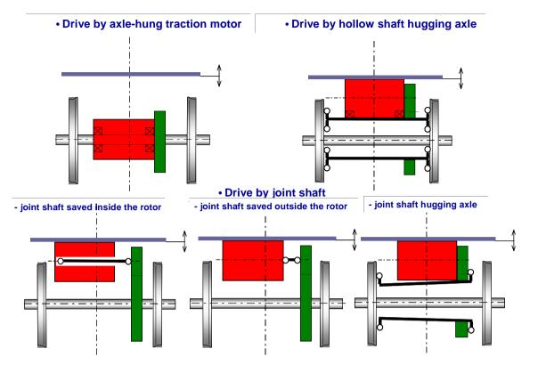
Fig. 1. The basic scheme of construction types of wheelset drive systems
