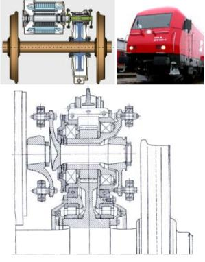
Fig. 5. System RHA – joint shaft inside hollow pinion loc. 2016 series (Hercules) and a detail section
