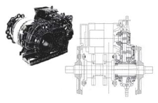
Fig. 9. Integrated drive QIH 5018 (Bombardier), used at locomotives 412 and 101 series
