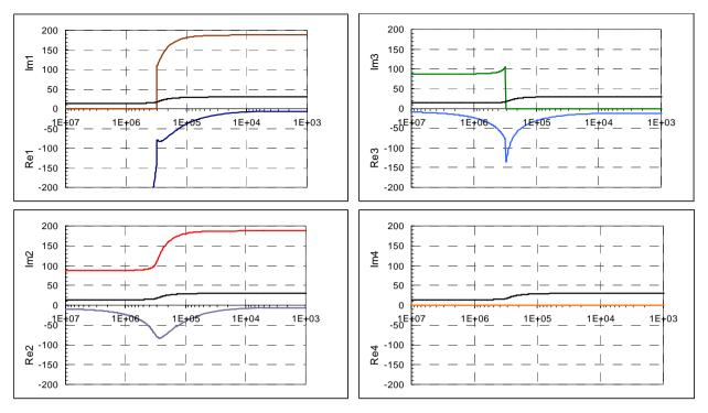
**Fig. 26.** Courses of eigenvalue roots of system before and after steep start (crossing through the adhesion characteristics peak)
