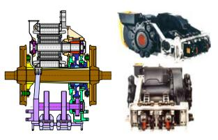
Fig. 8. Integrated unit HAB with additional brake shaft (Siemens 1016/1116 – Taurus)
