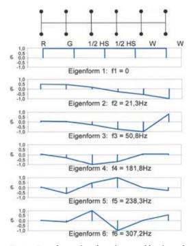
Fig. 25. Eigenform values for 6 degrees of freedom of torsional models of Eurosprinter wheelset drive
