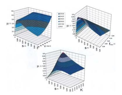
Fig. 14. The 3D-dependences of adhesive characteristics on drive speed, friction coefficient and steepness
