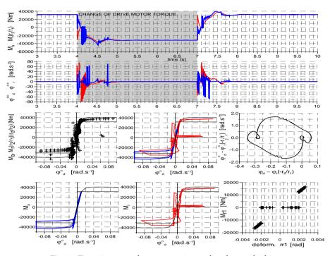
Fig. 24. Transition action between traction work and motor braking
