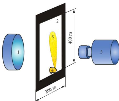
Figure 2. Optical measurement scheme and screen design: 1 – lamp; 2 – scattering screen; 3 – fuel jet; 4 – nozzle; 5 – high-speed video camera
