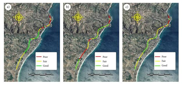
Fig. 3. Design consistency evaluation according to Lamm's *safety criterion I*: a – North–South direction; b – South–North direction; c – both directions
