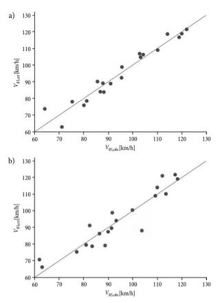
Fig. 5.  $V_{85,est}/V_{85,obs}$  for curves (a) and tangents (b)
