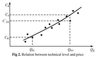
This curve can be used for evaluation of general (overall) efficiency of video cameras. Consequently selection efficiency of particular video camera [6] is expressed as:
