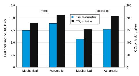
Fig 7. The relationship between average fuel consumption and  $CO_2$  emission of an automobile and type of transmission used
