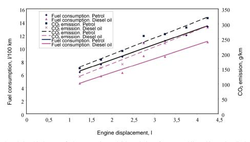
Fig 4. The relationship between fuel consumption and CO<sub>2</sub> emission of an automobile and its engine displacement
