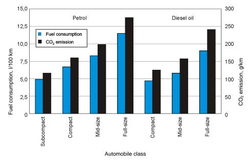
Fig 6. The relationship between average fuel consumption and CO<sub>2</sub> emission of an automobile and its class
