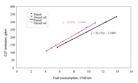
Fig 2. The relationship between CO<sub>2</sub> emission and fuel consumption of a motor car
