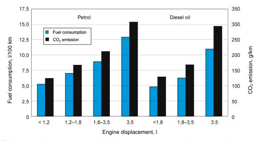
Fig 3. Average fuel consumption and CO<sub>2</sub> emission by a motor car depending on its engine displacement
