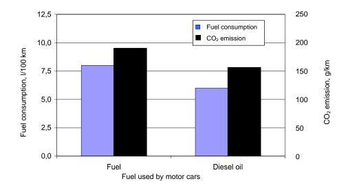
Fig 1. Average fuel consumption and CO<sub>2</sub> emission by motor cars depending on the fuel used
