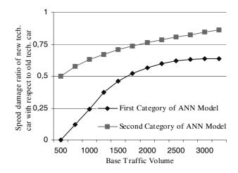
Fig 4. Speed damage ratio of two wheeler w. r. to old tech. car at different base traffic volumes
