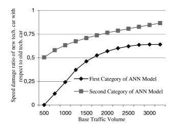
Fig 3. Speed damage ratio of new tech. car w. R. to old tech. car at different base traffic volumes
