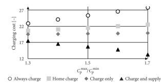
Figure 11. Charging cost of daily routine as a function of electricity rate fluctuation when  $(C_s/C_p = 0.95)$
