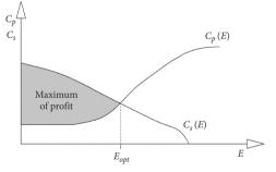
Figure 9. Maximum of profit of supply mode if the amount of energy of sections converges to 0
