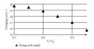
Figure 12. Charging cost of daily routine in case of charge and supply mode as a function of the rate of  $C_s$  and  $C_p$  $\left(C_p^{\max}/C_p^{\min}=1.5\right)$
