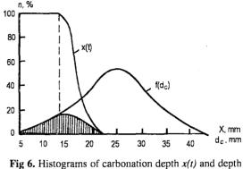
Fig 6. Histograms of carbonation depth x(t) and depth of rebar cover  $d_c$  in reinforced concrete bridge pier  $(f_c) = 20$  MPa; t = 30 years)
