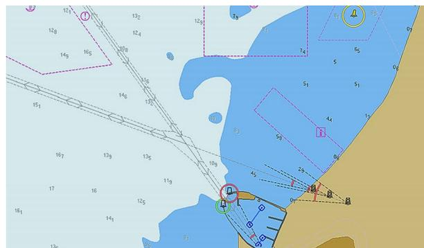
Figure 1. The approach channel to the Port of Ventspils (160 m in width)
