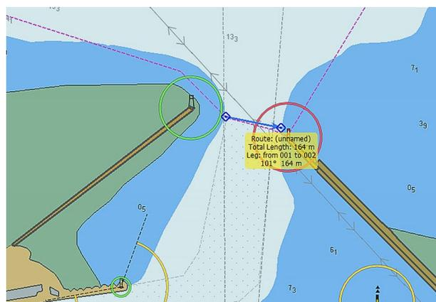
Figure 4. The approach channel to the Port of Dunkerque (width of the port gate is 164 m with a short area for ship stopping)
